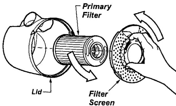
Grasp primary filter, rotate counter-clockwise and lift out. Clean primary filter by gently tapping over a trash container.
